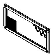
Caution should be used on both filters to ensure the sealing panel on the rear of the filter is not damaged. In the case of damage, the filter should be replaced immediately.
